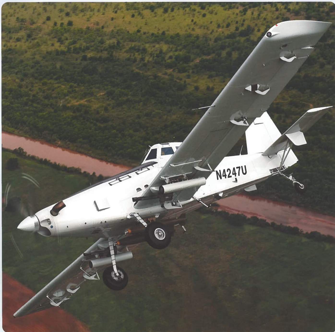
An Air Tractor AT-802U in flight. The plane is essentially a two-seat combat-ready crop-duster with weapons and advanced electronics. Photo courtesy of Air Tractor, Inc. Olney, TX
